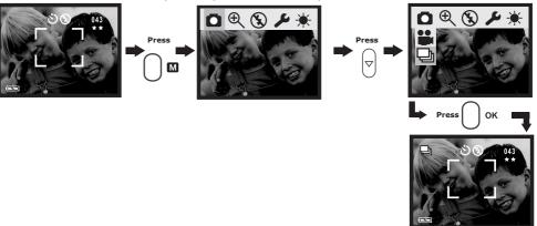
When the above setting is done, Icon 🖃 appears on LCD screen, hold down the Shutter button to record continuous pictures. You can capture 4 pictures in continuous pictures mode.
