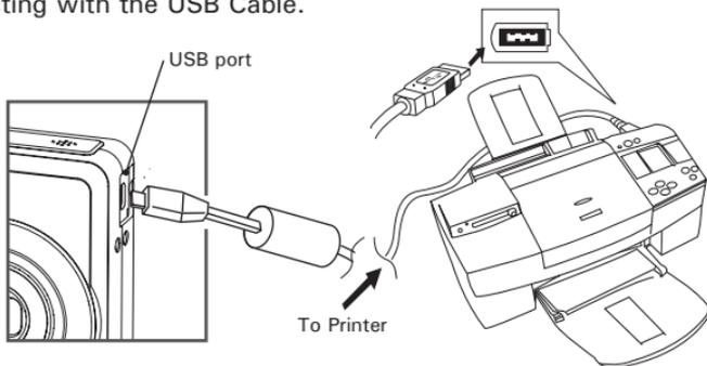
1. Plug the labelled end
