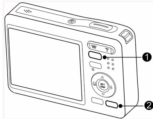
In PLAY mode, press the **PLAYBACK** (❶) or the **MODE** (❷) button to switch to the REC mode.
