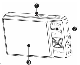
Press the POWER button (1) again to turn the power off.
